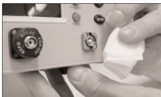
Figure 13. Cleaning the ferrule in the connector port
