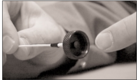
Figure 7. Cleaning the FOA
