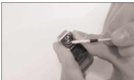
Figure 11. Cleaning the EUI
